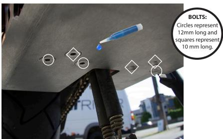
Pivot the rear of the skid plate into alignment with the rear brackets. You may need to loosen bracket bolts to allow enough play to get the correct alignment. Start the (6) M8 flat head bolts using an M5 allen driver. Once all installed, torque them to 10 nm. Use thread locker.
